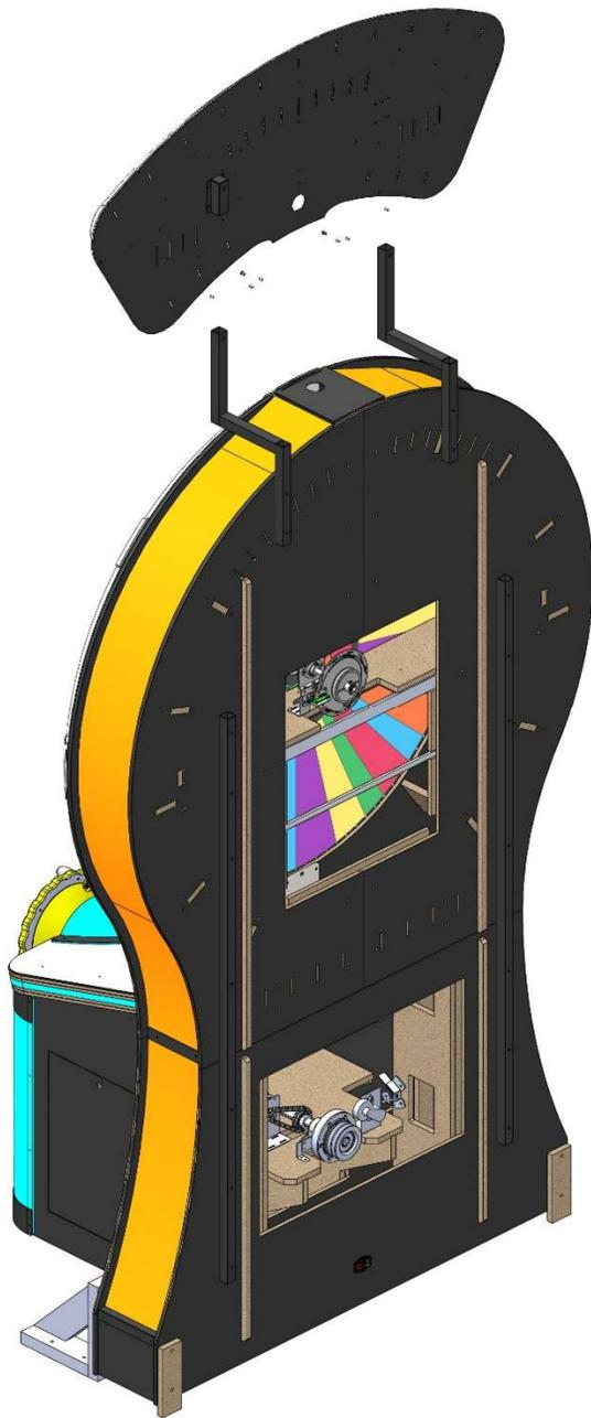
**STEP 8: ATTACH HAT BRACKETS TO MARQUEE WITH 8X #8-32 X .375L SCREWS**
