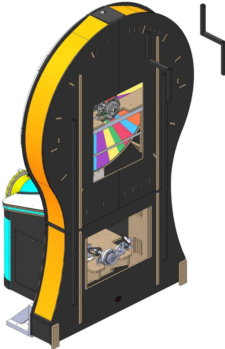
**STEP 7: INSTALL MARQUEE SUPPORT TUBES WITH 4X ¼-20 X 2.000L SCREWS**
